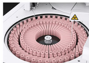
Reagent Tray 2~8°C cooling for 24 hours.
