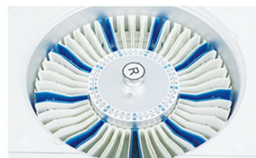
Reagent Tray 2~8°C cooling for 24 hours.
