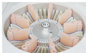
Reagent Tray 2~8°C cooling for 24 hours.
