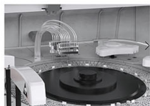
Reaction Tray 37±0.1°C, water bath.
