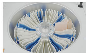
Reagent Tray 2~12°C cooling for 24 hours.
