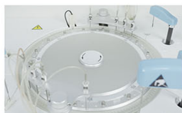
Reaction Tray 37±0.1°C, water bath.
