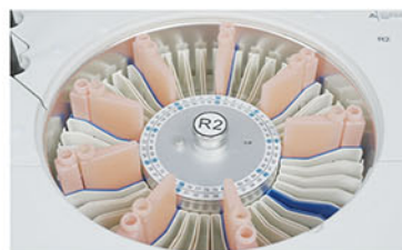
Reagent Tray 2~8°C cooling for 24 hours.
